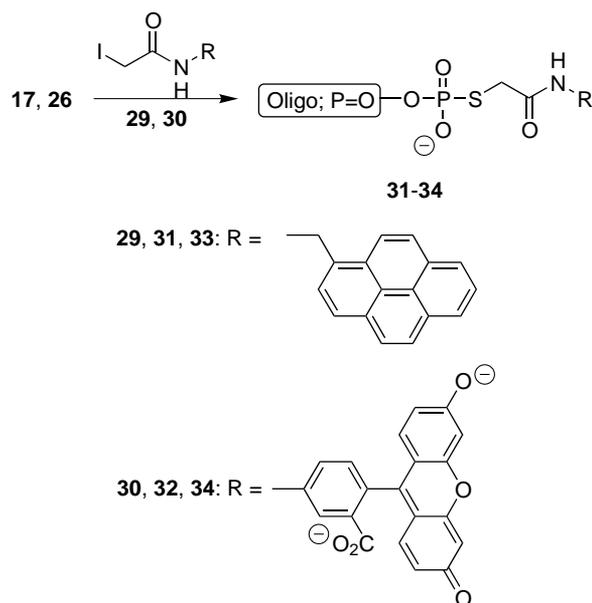
**Scheme 4.** For **17**, **31** and **32**: Oligo = 5'-pS-ATGCAT<sub>2</sub>CTGC<sub>5</sub>A<sub>2</sub>G<sub>2</sub>A-3'; for **26**, **33** and **34**: Oligo = 5'-TGCATC<sub>5</sub>AG<sub>2</sub>C<sub>2</sub>AC<sub>2</sub>AT-pS-3'.
